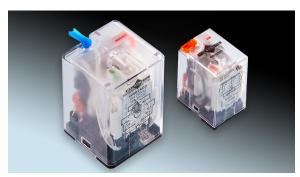
General Purpose Relays are designed for easy installation, testing and troubleshooting. Push-to-test buttons are color coded – orange for AC and blue for DC voltage coils. The buttons can be locked in place for testing. LED lights provide confirmation that the relay is energized.
