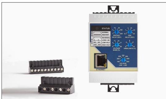
Compact 60 mm wide enclosure mounts on DIN-rail or can be panel mounted with two screws inserted through clips that extend from the back of the enclosure. Pluggable terminal blocks on both the inlet and output side enable easy installation and replacement without removing any wires.
