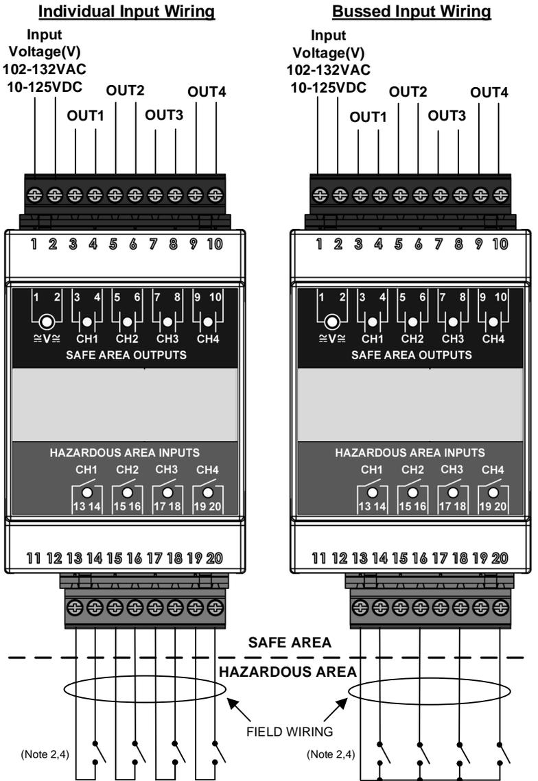
(Separate terminals are provided for connection of two conductors per channel. Use of all channels is not required. Individual, bussed, or a combination of input wiring configurations may be used.)
